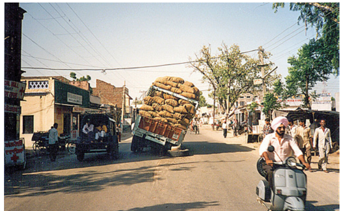
Figures 24 and 25: Overloading is a major cause of crashes. The front wheels of a truck loaded with bamboo trunks in Bangladesh (top) barely touch the ground, while a grossly overloaded truck in Amritsar, Punjab, India is a serious hazard.
